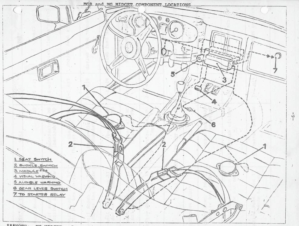
\*\*\*NOTE: MG MIDGET - Control unit is located on Bulkhead in Glove Box COMPONENT LOCATIONS
